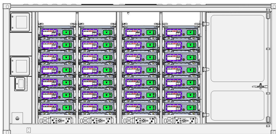
Figure 8 Front view of battery rack
